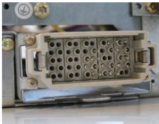
Control circuit terminals, up to 50 poles
