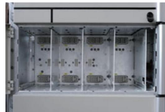
Q-type compartment, 4 module height to accommodate 4 Q-type extractable units with power-side protective contacts and load-side insulating contacts
